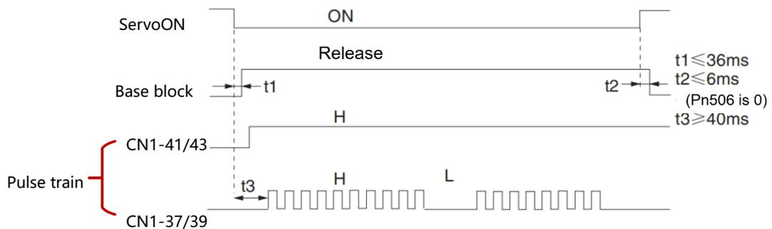
Set the time interval (t3) from the servo ON to the start of pulse train command input to 40ms or more. If the input is within 40ms, the servo unit may not be able to receive command pulses.
