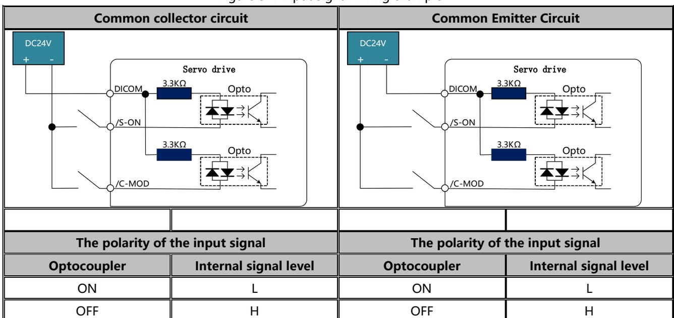
Users can assign the input signals through Pn500~Pn505 include: /S-ON (servo ON), /C-SEL (control mode switching), P-OT (forward side drive prohibited), N-OT (reverse side prohibited) drive), /CLR (position deviation clear), /ALM-RST (alarm reset), /G-SEL (gain switching), etc.
