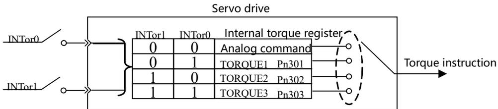
Note: After selecting the external input signal as INTor1 and INTor0, if the INTor1 and INTor0 signals are not input, the selected torque is "external analog command" (00. 01), the torque value is Pn301.
