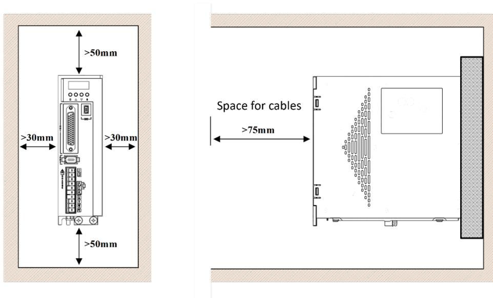
When installing multiple drives in the control cabinet, ensure the spacing shown in Figure 2-4.
