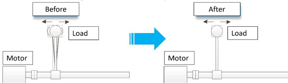
This function is based on model tracking control. According to the relationship between the load position and the motor position in the model loop, in order to control the position stability of the load end, the position command of the motor end is corrected, and the feedforward value generated by the model is corrected to achieve low-frequency vibration suppression. the goal of. Its working schematic is shown in Figure 9-34.
