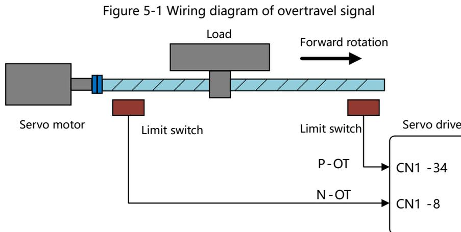
When the driver is used for rotating loads such as round tables and conveyors, it is usually not necessary to use the overtravel prevention function. In this case, it is not necessary to wire the input signal for overtravel prevention.
