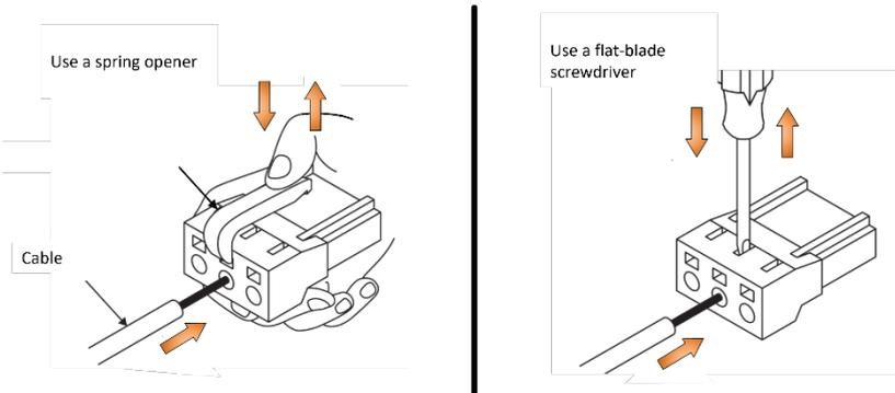
Step 9 After the wiring is completed, install the main circuit connection terminal and the control circuit connection terminal to the connector of the drive.
