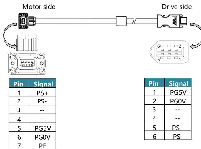
►LQ1-E0B0-□□ (Encoder cable with battery)
