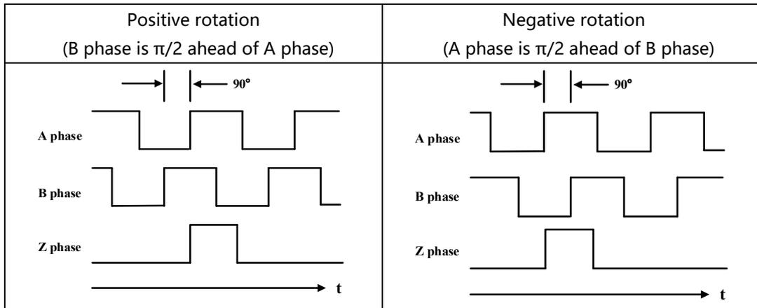
Please rotate the servo motor by two turns before using servo drive Z phase pulse output for mechanical reference point reset action.
