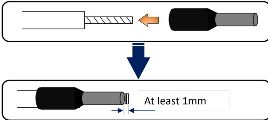
Step 4 Use wire pliers to compress the wire with the ferrules and trim the exposed wire ends.
