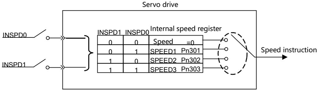
Note: After selecting the external input signals as INSPD1 and INSPD0, if the INSPD1 and INSPD0 signals are not input, the selected speed is "speed=0" (00); if the INSPD0 signal is valid and the INSPD1 is invalid, then "SPEED1" (01) is selected. , the speed value is Pn301.
