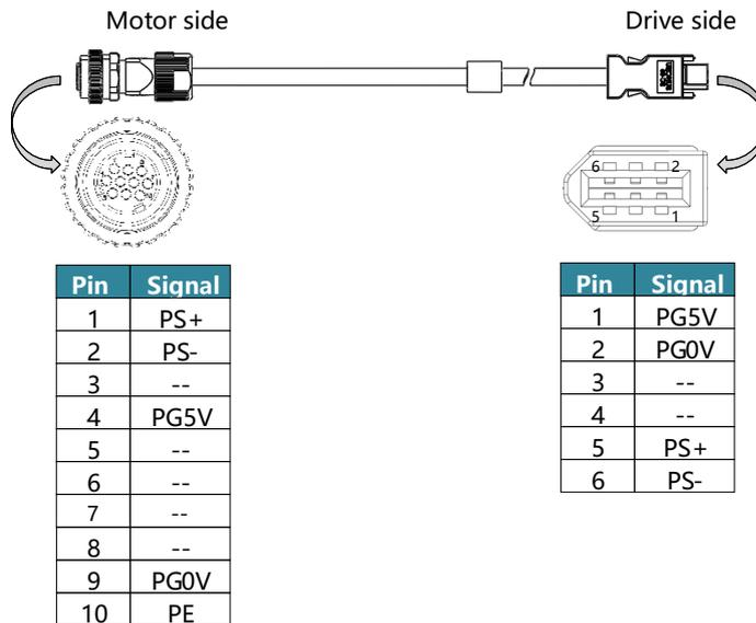
►LQ1-E0B2-□□ (Encoder cable with battery)
