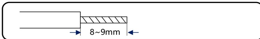
Step 3 Insert the core of the wire into the cold-pressed terminal (the core should be exposed at least 1mm from the cold-pressed terminal).
