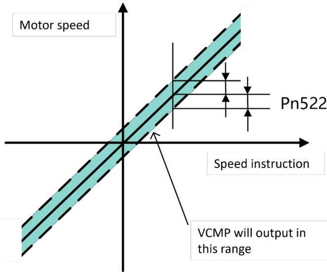
For example, Pn522=100, speed instruction is 2000rpm, if motor speed is within 1900rpm to 2100rpm, VCMP will be ON.
