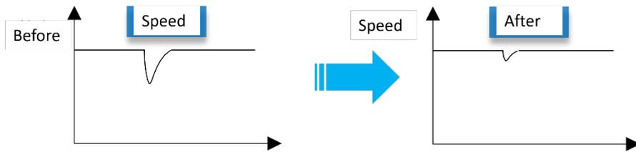
The load torque compensation function is to observe the load torque through the load torque observer, and then compensate the torque to the torque given, so as to achieve the effect of load torque compensation.
