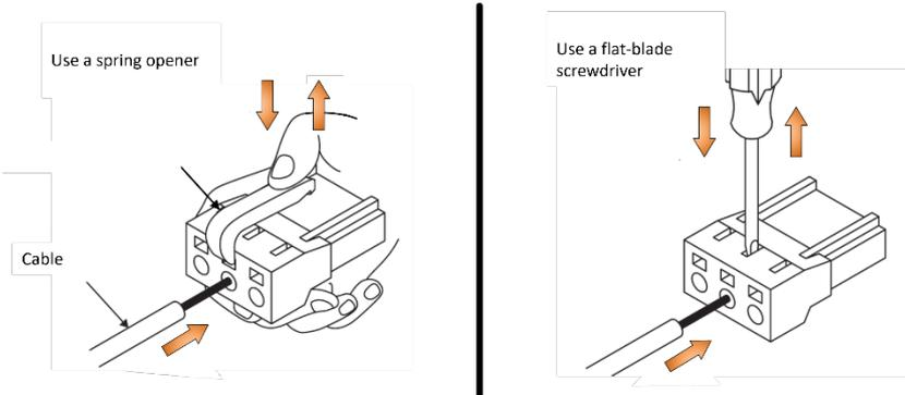
Step 6 With the wires inserted into the terminals, pull out the spring splitter or flat-blade screwdriver.
