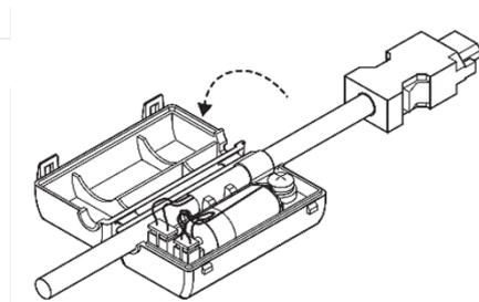
Step 3 Remove the old battery and install the new one.
